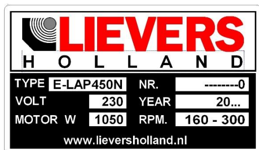
Fig 1: Type plate E-LAP450N The type plate can be found on the motor.
